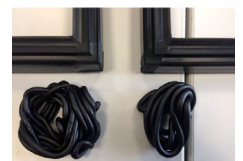
Comparison injection compound 90° left / 50° right
